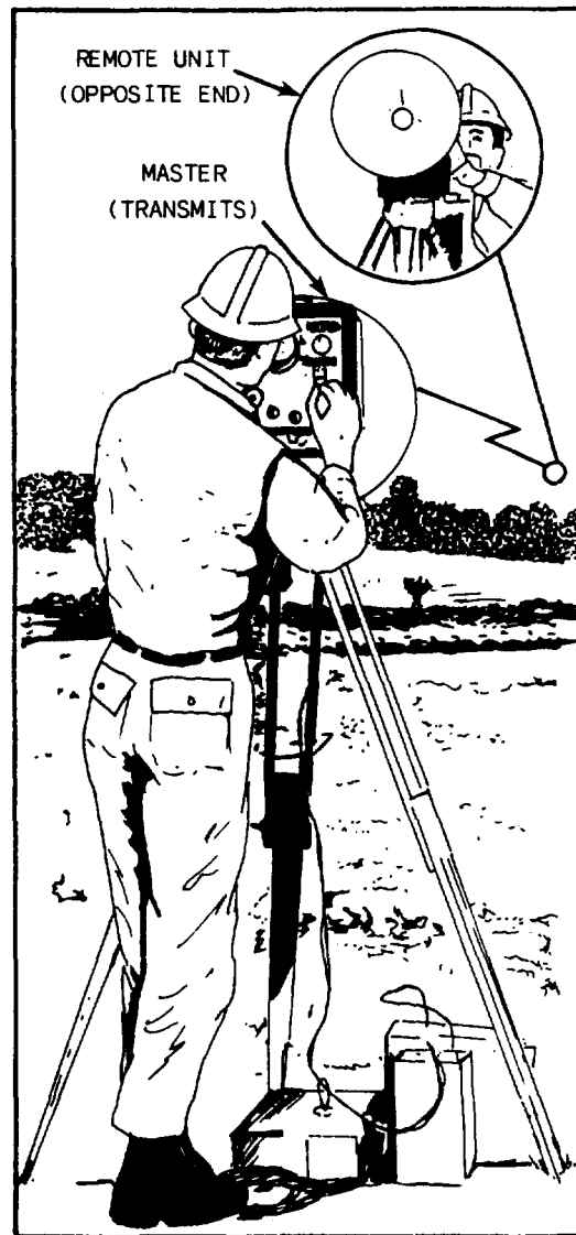
Figure 12-24. Setting a microwave distance-measuring unit.
